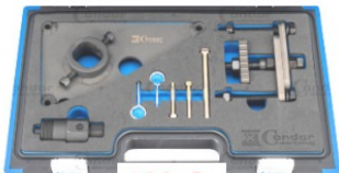
36901P Hyundai / Kia 1.1, 1.4, 1.5, 1.6 and 1.7L Common-Rail diesel. D3FA, D4FA, D4FAH, D4FAL, D4FB, D4F BH, D4FBL, D4FC, D4FD, D4FDH, D4FDL
